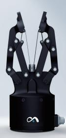
Flexiv's revolutionary force-controlled robotic gripper series Grav includes two gripper models: Grav and Grav Enhanced. Featuring Flexiv's industrial-grade force control and an adhesive material based on a gecko's foot pad, Grav is capable of picking up or manipulating practically any object that fits within its grasp.
